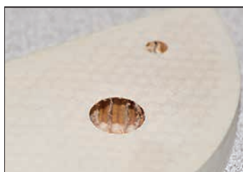
Hole for Fastener Produced with 34-100 Series
